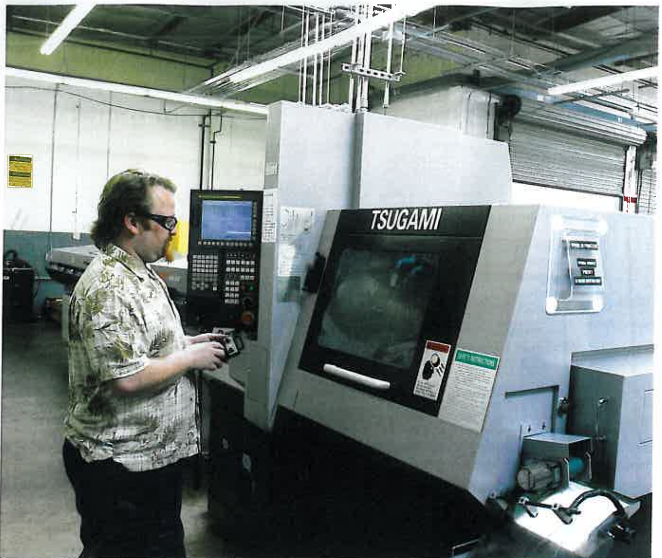
Corey Bryant, lead machinist for Submersible Systems, sets up a Tsugami Swiss-style turning center equipped with live tooling and a bar feeder. The Tsugami is designed specifically for short cycle times and was purchased to cut production costs on the Spare Air and to eventually allow the company to bring in outside "job shop" work. The system features a Fanuc 31i-A dual path CN controller and 8,000-rpm main and subspindles for high-speed turning and reduced cycle times. The Spare Air product is CE certified and Submersible Systems, Inc. is currently undergoing ISO certification.
