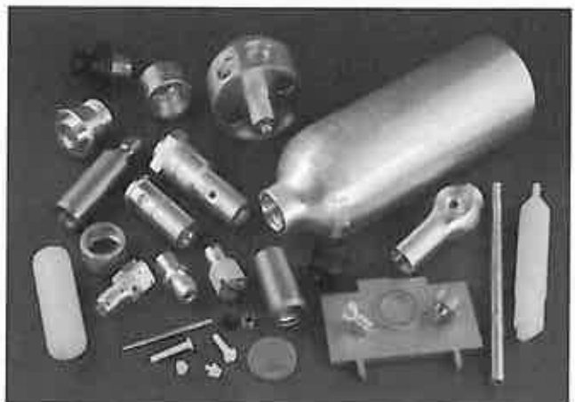
Some of the parts that are produced to manufacture a Spare Air breathing system. 22 of the parts are now fabricated in house.
